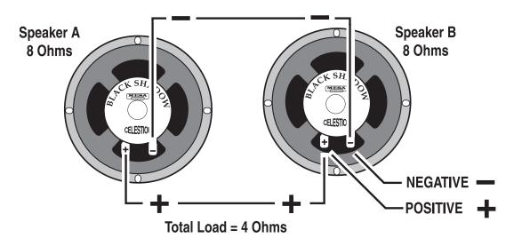
COMBINATION OF SERIES & PARALLEL: This is really just two sets of Series wired speakers connected in Parallel. This is how you maintain a consistent load with multiple speakers. The importance of this is more evident when you have more than one cabinet to connect to your amplifier. This is when you need to figure out the loads and how to wire them up without applying too low of a resistance on the amplifier.
