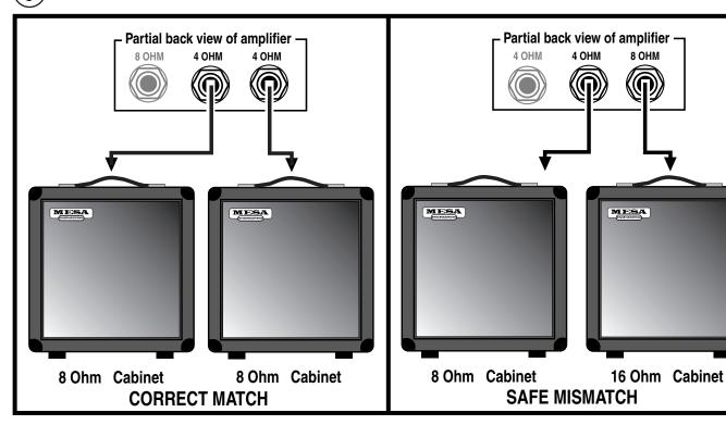
8 (9) Partial back view of amplifier -Partial back view of amplifier -4 OHM 4 OHM 8 ОНМ 8 OHM 4 OHM 8 Ohm 8 Ohm **PARALLEL BOX SERIES BOX CORRECT** 4 Ohm 16 Ohm 4 Ohm 16 Ohm **CORRECT MATCH MATCH** MESA MESA MESA MESA 4 Ohm Cabinet 4 Ohm Cabinet 16 Ohm Cabinet 16 Ohm Cabinet
