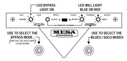
However, the Normal configuration works great if you need an alternate clean sound of a different level and tone. The Normal position can also work great for driving an amplifier's front end stage into clip by using the Clean mode and setting V-TWIN'S Gain control high and switching it in for the *pushed* rhythm sound or a lower gain Solo sound.
