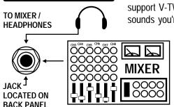
This 1/4" output and its accompanying switch (located on the side panel) support V-TWIN's recording circuit. This circuit is voiced to re-create the sounds you're accustomed to hearing from the "To Guitar Amp" and "To
