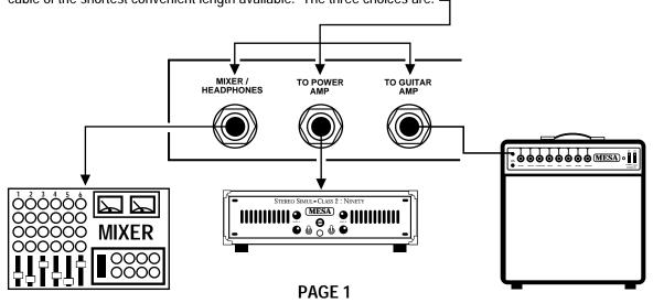
BASIC SET-UP: Set the controls as per this diagram. Then run through the 3 sounds by using the Channel Select footswitch and the Alternate Channel push key located between the Middle and Treble controls.
