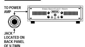
interfacing with the *FX Return* stage of any amplifier, or simply to use V-TWIN as a stand alone pre-amp with an existing power amplifier. (We suggest an all tube power amp...e.g. MESA'S *Stereo Simul-Class 2: Ninety* or *Fifty/ Fifty.*)
