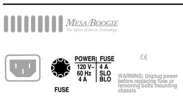
If you see nothing abnormal as you lift the STANDBY switch, it is possible that a power tube shorted temporarily and blew the Fuse. If this is the case it may work again normally. To be safe, you might want to replace it and just the adjacent tube or all power tubes in the “shotgun” troubleshooting tradition and save the replaced set as spares. Spare fuses are a must for the
