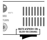
NOTE: When this switch is set to the "ON" position, a speaker load must be maintained by either a load resistor of some type or a speaker itself. Failure to comply with this instruction could result in major damage to the amplifier. Leave your speaker connected.
