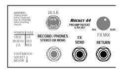
When the RETURN is used as an input, the ROCKET 44's MASTER controls are the only two controls being utilized regardless of which one of the three modes you happen to be in. Also, while the RETURN is being used in this manner, all other controls are inactive.
