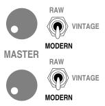
The added tightness of the low end response combined with the radically more present top end keeps the MODERN mode tracking accurately even at extreme gain settings. Keep in mind that when using MODERN in CHANNEL 3 you will have to run the PRESENCE control almost all the way up to approach the lower range of the PRESENCE control in CHANNEL 4.
