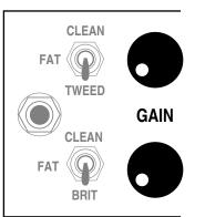
In most guitar amplifiers, and especially in all-tube circuits, the GAIN control is the most powerful control in the preamp. It shapes the overall style and character of the sound and is responsible for whether the sound is clean, overdriven or anywhere in between. In your **Road King**, the GAIN control is even more powerful. It not only determines the amount of drive, but also acts as an integral part of the tone control string as well.
