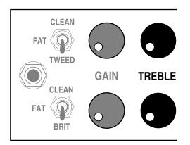
is very important for equal representation of the three frequency regions to appear at their respective controls. Like most of the controls on your **Road King**, there is an optimum region of the TREBLE control where ample top end is mixed in and yet enough signal is still passed on to the MIDDLE and BASS controls.
