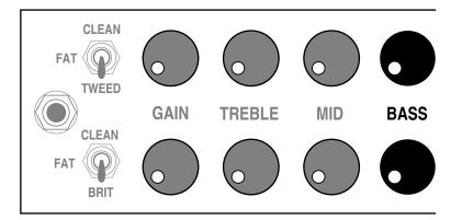
For the most balanced sound and a balance of power between the three rotary tone controls, try to use the TREBLE control in its middle ranges. This scenario produces nearly equal representation of all the frequencies on the tone controls and provides a great nuetral starting point for further tweaking.
