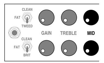
these MIDDLE control settings ( 2:00 - 5:00 ) can introduce added gain and create enhanced focus, the trade-off will be a stiffer, more forward, less compressed feel.
