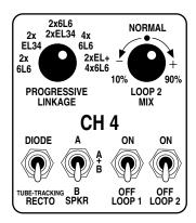
This section is where you choose the status of LOOP 1 & 2, your choice of Speaker enclosure(s), what type of Rectifier you wish to use and most importantly the power section you wish to combine with your preamp choice with the PROGRESSIVE LINKAGE rotary control. Let's go over the controls one at a time, beginning with this most important choice.
