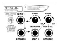
both LOOPS along with their controls, the Front Panel OUTPUT and SOLO controls and two 12AX7's are taken out of the circuit. This leaves the individual Channel MASTER controls as the main volume controls. Front Panel LED indicators for each Loop located between the pairs of Channels to keep you abreast of LOOP 1 & 2 status.
