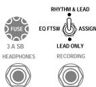
RECORDING: This jack provides direct-to-console interfacing for recording or sound reinforcement applications. It is a circuit dedicated to reproducing the roll off that occurs in the output section with a speaker connected. The send level strength is determined by the GAIN and MASTER controls. From the RECORDING jack, adequate signal level will be available for most of your recording needs and live performances.
