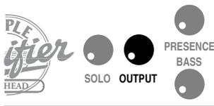
**NOTE:** When using the *EFFECTS RETURN* as an input - to use the *Recto* as a power amp - the *SOLO* Control can be used to attain a footswitchable boost if the Footswitch is connected. It is wired in parallel to the **OUTPUT** Control and therefore also controls the volume of the power section.
