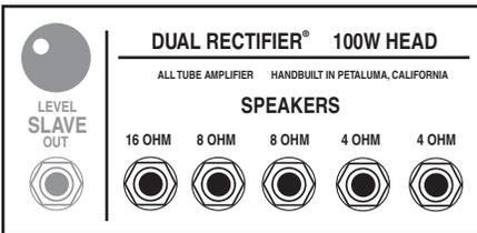
4x12 cabinets may be 4, 8 or 16 Ohms. If you are not sure of the impedance of your cabinet, you may need to remove the Rear Panel in order to verify the impedance rating of the individual speaker or speakers. *MESA/Boogie* 4x12 and 4x10 cabinets come standard wired to 8 Ohms, and are wired in series-parallel. Some Non-*MESA* 4x12 cabinets are wired 16 Ohms using four 16 Ohm speakers. By wiring all four speakers
