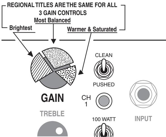
In most guitar amplifiers, and especially in all-tube circuits, the **GAIN** Control is the most powerful control in the preamp. It shapes the overall style and character of the sound and is responsible for whether the sound is clean, overdriven or anywhere in between. In your *Recto*, the **GAIN** Control is even more powerful. It not only determines the amount of drive, but also acts as an integral part of the tone control string as well.
