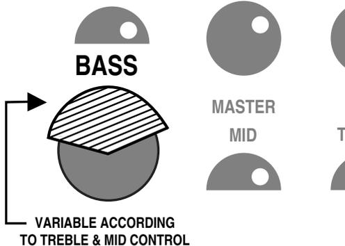
mixes in changes from channel to channel. Like the MIDDLE Control, it falls in line signal-wise *after* the TREBLE Control and the same scheme applies. When the TREBLE Control is set high, the effectiveness of the BASS and MIDDLE Controls is reduced. If the TREBLE Control is set low these two controls become dominant.
