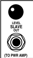
**NOTE:** Once a signal is taken from the **SLAVE**, it can not be inserted back into the FX Loop Return jack or a feedback loop will occur. Much like holding a microphone into the PA system's cabinets...a loud high pitched squeal will be the result.
