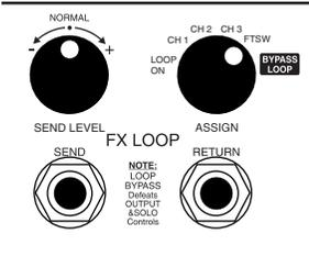
1.) An **ASSIGN** rotary control that allows you to have any combination of LOOP ON status or completely remove it from the signal path altogether.
