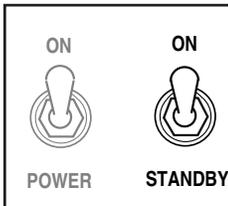
Wait at least 30 seconds and then flip the **STANDBY** switch to the ON position. This prevents tube problems and increases their toneful life substantially.
