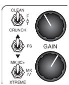
In both the Channels, there are three regions of the GAIN control. A low gain zone between 9:00–11:30, a warmer, more saturated zone from 12:00–2:00 and a higher gain zone from 2:30–5:30. Each of these zones can be used for many different applications and all can be used for both chording and single note solo work. As the GAIN control is swept throughout its range it imparts different textures and tonal characteristics.
