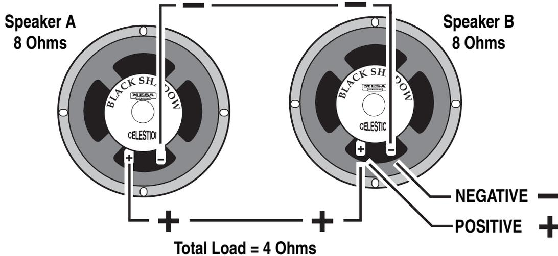
**COMBINATION OF SERIES & PARALLEL:** This is really just two sets of Series wired speakers connected in Parallel. This is how you maintain a consistent load with multiple speakers. The importance of this is more evident when you have more than one cabinet to connect to your amplifier. This is when you need to figure out the loads and how to wire them up without applying too low of a resistance on the amplifier.
