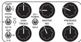
**CLEAN** is derived from a blend of our best MARK series clean sounds taken from the MARK IV and is perfect for rhythm comping in an ensemble environment where the guitar has to fit in a defined spot in a more complex mix. It is also extremely accurate in the time domain and has a balanced blend of tight low end to the sparkling, immediacy of the top end. This mode also clips great in the 45 and 10 watt power modes with its' well balanced, more stripped nature.
