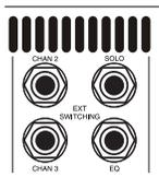
The **EXTERNAL SWITCHING** jacks override the *MARK V*'s Foot controller. Once a Channel or Feature has been triggered "On" at the EXT. Switch ports, it may not be controlled or turned "Off" until the logic at the Switch Port is reversed.
