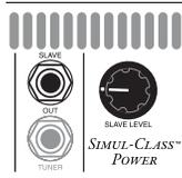
**NOTE: Once a signal is taken from the SLAVE, it can not be inserted back into the EFX Loop Return jack or a feedback loop will occur. Much like holding a microphone into a PA system's cabinets...a loud high pitched squeal will be the result.**
