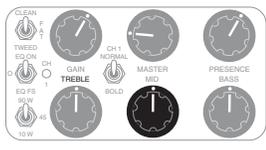
For rhythm playing in the *CLEAN* and *FAT* Modes of Channel 1, a lower *MID* setting (7:30 – 10:00) scoops some of this midrange attack and makes the bottom end breathe more. This range will also make things more resilient and create an easier to play, more elastic feel on the strings. Single coil guitars work very well here for the slinky, rubber band attack and bouncy bass character associated with Blues, R&B and Country clean styles.
