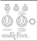
**NOTE:** The MUTE and EFX LOOP only are active when the EFX LOOP is in LOOP ACTIVE (toggle up) Mode.
