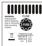
If you see nothing abnormal as you lift the STANDBY switch, it is possible that a power tube shorted temporarily and blew the **FUSE**. If this is the case it may work again normally. To be safe, you might want to replace just the adjacent tube or all power tubes in the "shotgun" troubleshooting tradition and save the replaced set as spares. Spare fuses are a must for the fabled cord bag along with your spare tubes. Always carry both for they could be worth their weight in gold someday.
