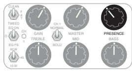
You can think of the PRESENCE as a control that allows you to either clamp the power amp down, compressing it and darkening things - or open it up and let the full spectrum of upper harmonics come blazing through. It also has a great deal to do with how dynamic the signal is and how a sound will cut through the mix in an ensemble environment.
