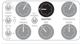
For you purists... when the EFFECTS LOOP is set to the HARD BYPASS (toggle down) setting on the Rear Panel, the MASTER control becomes the final volume control (because the OUTPUT level control is part of the EFFECTS LOOP circuitry). To raise or lower the playing level of the entire amplifier, you
