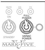
**FULL POWER** supplies the amplifier with the full 120 volts of voltage (depending on line conditions at any given time) and produces the maximum volume, headroom and punchy bold tone throughout the Channels.
