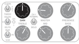
In all the Channels, there are three regions of the GAIN control – a low gain zone between 9:00 - 11:30, a warmer, more saturated zone from 12:00 - 2:00 and a higher gain zone from 2:30 – 5:30. Each of these zones can be used for many different applications and all can be used for both chording and single note solo work. As the GAIN control is swept throughout its range it imparts different textures and tonal characteristics.
