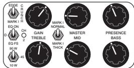
**EDGE** is the lowest gain Mode in Channel 2 and is EQ'd to be stripped, urgent and fast. Low end is tucked up higher and reduced slightly to increase dynamic response and increase attack speed. Works extremely well for classic Rock broken-up chording sounds in the medium GAIN range. GAIN set high produces articulate, biting single note sounds.
