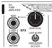
**NOTE:** The Front Panel OUTPUT and SOLO controls are both part of the Loop and therefore active only when the Effects Loop is engaged. They are both part of the Return stage and will remain inactive as long as the loop bypass mini toggle is set to HARD BYPASS.
