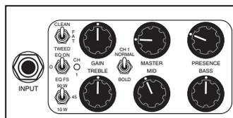
The medium gain TWEED Mode (switch down) is dedicated to pushed, overdriven “clean” sounds. TWEED increases gain in the low mids and adds fatness which creates a smoother sound when clipped. This added gain slows the attack a bit but in turn adds sustain and girth. A balanced dynamic content makes TWEED work equally well for both broken-up chording and urgent single note soloing.
