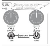
Rectifiers are selected automatically (Solid State) in the 90 Watt and (Tube) in the 10 Watt Modes according to their power requirements and associated sound styles.
