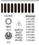
**NOTE: It is extremely important that the BIAS SWITCH setting match the type of tubes in use. Failure to comply will result in damage to your amplifier. Always check the BIAS SWITCH whenever swapping tubes!**
